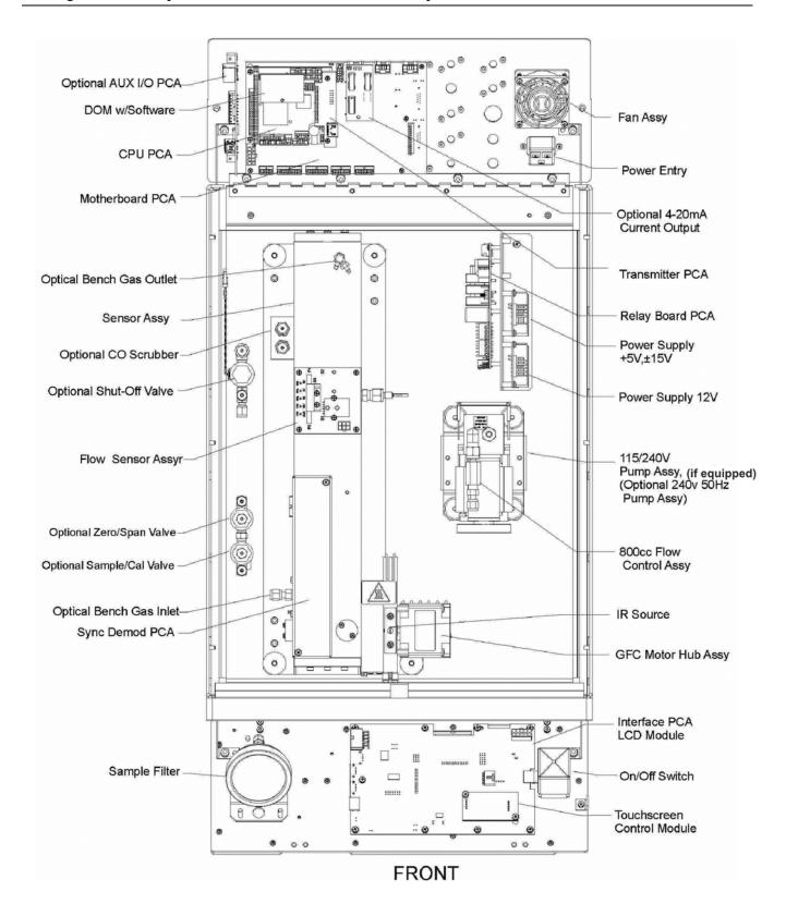
Figure 3-5: Internal Layout – GFC7001T
